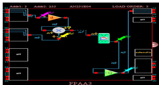
Fig.4. FPAA configuration for frequency demodulator (input is given from modulator circuit)
