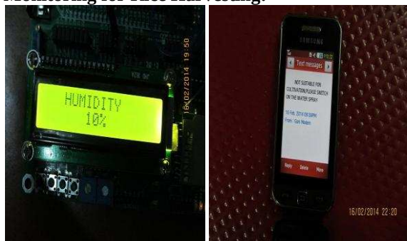
"Fig.10 Outputs for HSM20g sensor on LCD & Mobile Phone"
