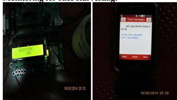
"Fig.13 Outputs for Soil Moisture sensor on LCD & Mobile"
