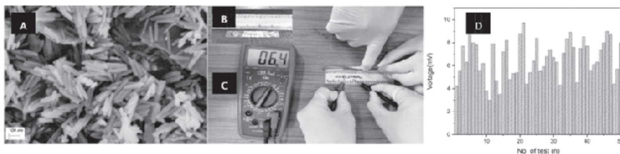
Fig. (A) ZnO nanorods, (B) Piezoelectric device, (C) Device testing, (D) Reliability test.
