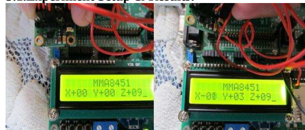
Fig.6 "accelerometer values at different head positions"
